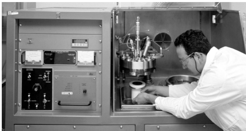
Dr Ulf Kreher, a postdoctoral fellow, assembling the reaction vessel of the custom designed microwave batch reactor which allows continual monitoring of temperature and pressure, removal of samples for monitoring and rapid well-controlled cooling via a cold-finger.
