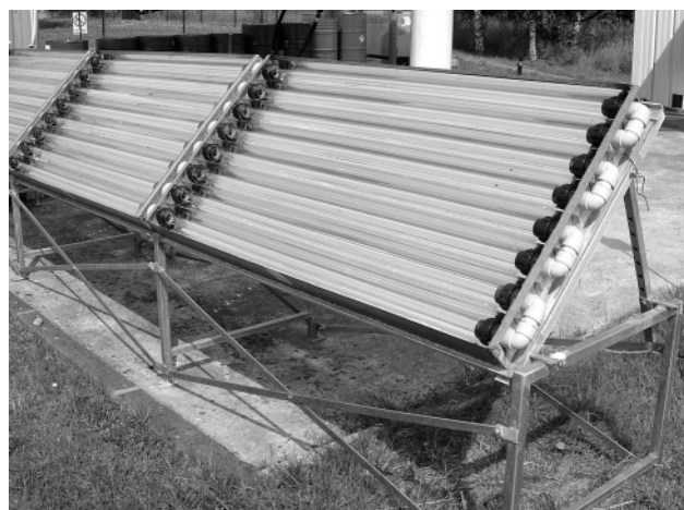
Fig. 3 CPC reactor with 3 m 2 reflecting area.
