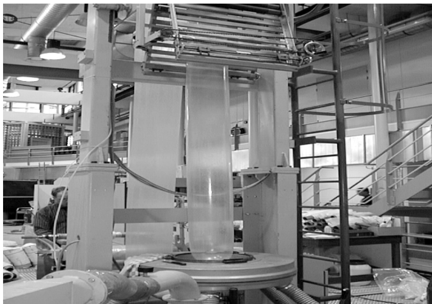
Fig. 2 Film blowing of co-extruded biopolymer multi-layered films.
