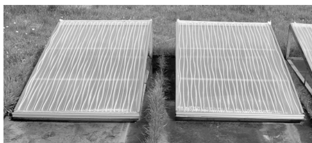
Fig. 4 Flat bed reactor with 3 m 2 of total reflecting area.
