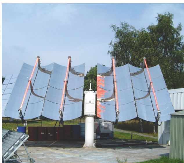
Fig. 2 The PROPHIS reactor. The building for the feeding platform can be seen in the background. Only one trough (3 m 2 reflecting area) was used for the experiment, and the brown–yellowish color of the photosolution can be clearly seen in the absorber tube.
